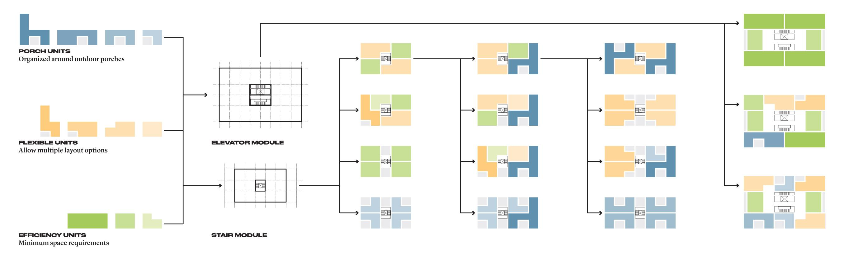
The number of structural bays can expand and contract in order to accommodate a variety of unit types and configurations
